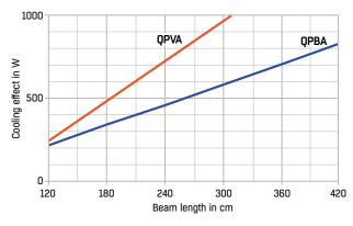
The diagram shows the approximate cooling effect,  $P_{tot}$  in W with water flow,  $q_w = 0.05$  l/s difference between room air temperature and average water temperature = 8 °C and max sound pressure level  $L_{A10}$  = 30 dB(A).
