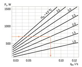
Correction for water flow, on basis of the diagram "Correction of cooling effect for water flow other than 0.05 I/s" is obtained K =  $P_{c \ 0,083}/P_{c0,05}$  = 1,05. The actual effect is therefore 5 % higher than the result given by the diagram, due to the higher water flow.  $P_c = 1,05 \times 218 = 229$  W/m
