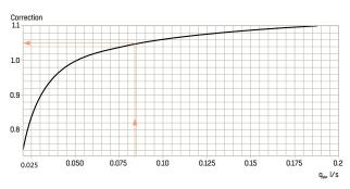
Required effective length (coil length)  $L_{eff}$  = 700/229 = 3,1 m. Casing length L = 3,1 + 0,1 = 3,2 m.
