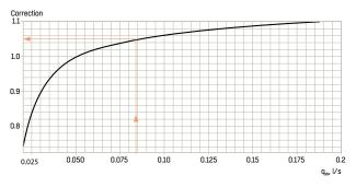
CORRECTION OF COOLING EFFECT FOR WATER FLOWS OTHER THAN 0.05 I/s
